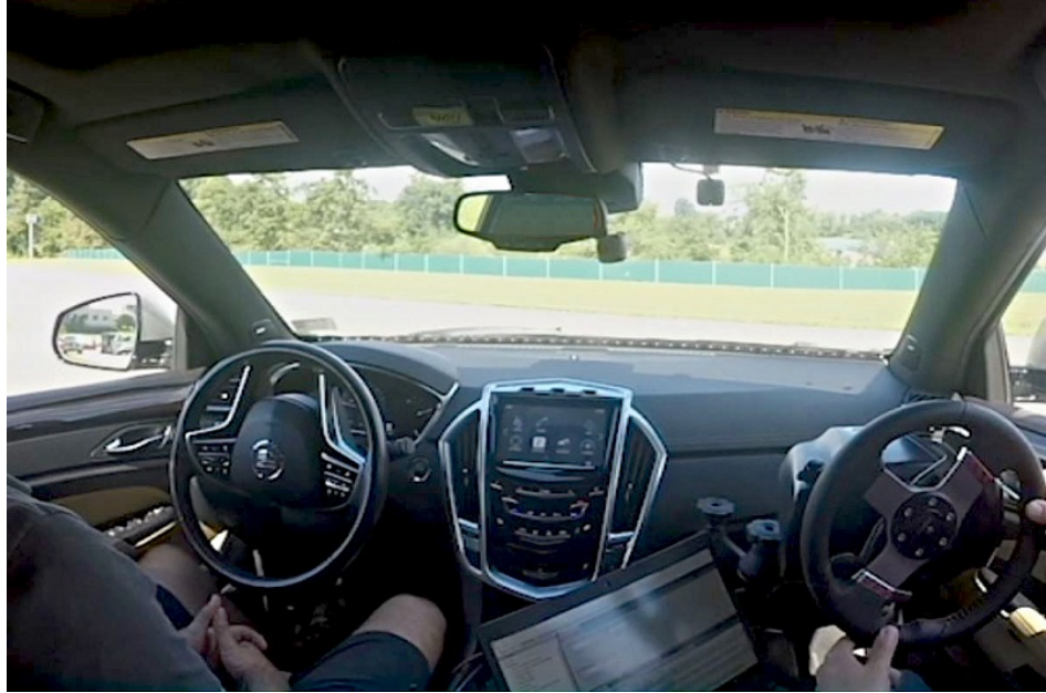
Figure 9. Test Platform to Execute FMVSS No. 114 via Human Control Method
